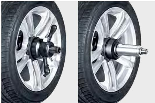
**Option 2: Flange:** mechanical or pneumatic wheel clamping
