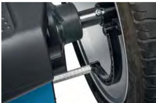
**The electronic data arm** determines the rim distance/ diameter and the position of the adhesive weights
