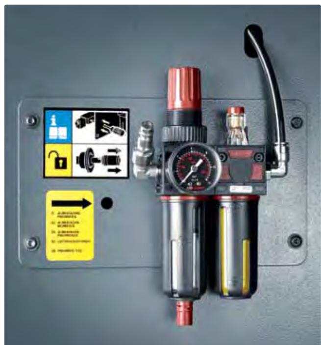
Service box: manual unlocking and compressed-air connection to the service unit (only in case of pneumatic flange)
